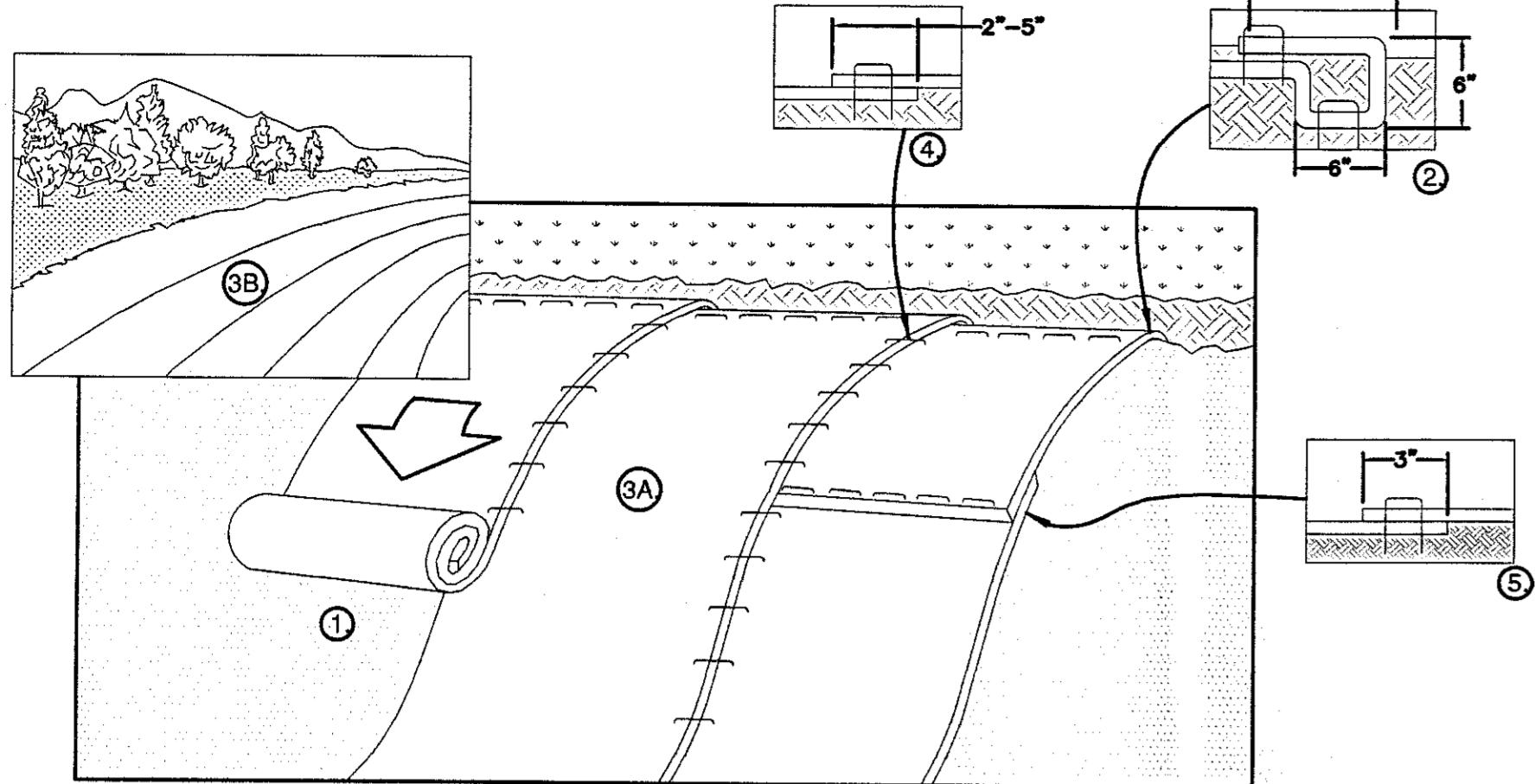
1. PREPARE SOIL BEFORE INSTALLING ROLLED EROSION CONTROL PRODUCTS (RECP's), INCLUDING ANY NECESSARY APPLICATION OF LIME, FERTILIZER, AND SEED.
