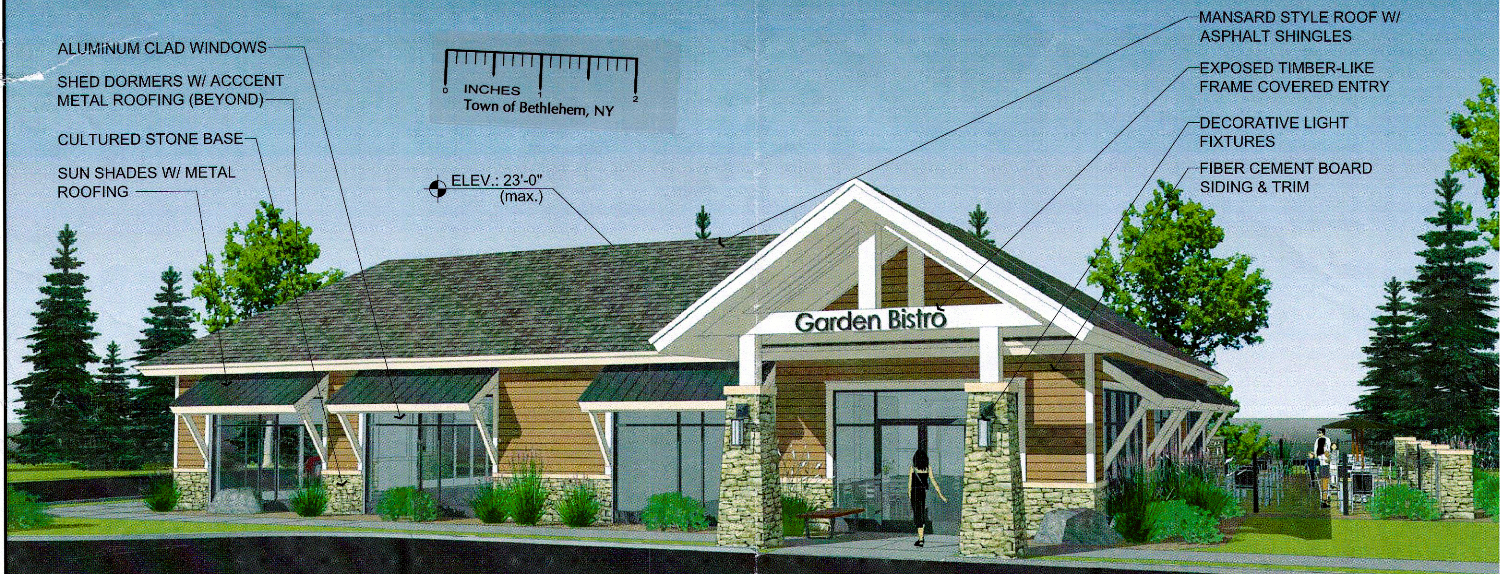
NORTH ELEVATION (SIDE)
