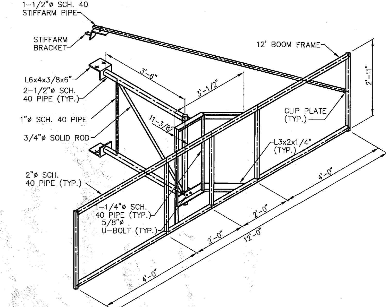
NOTE: BOOM ASSEMBLY ABOVE IS SHOWN AS PROVIDED BY: D&D WELDING, 4710 ROUTE 104, WILLIAMSON, NY 14589, (315) 589-4700. COORDINATE CONNECTION POINT TO TOWER WITH D&D WELDING PRIOR TO ORDERING.
