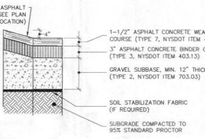
8 8 ASPHALT CONCRETE PAVING SECTION
