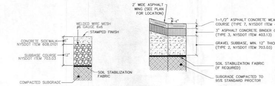
8 8 CONCRETE PAVING SECTION
