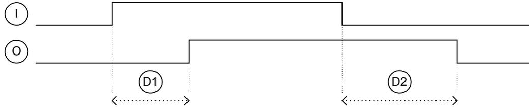
This option will delay the input to the output signal.
