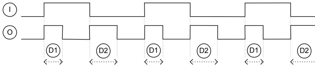
This option will create pulses on the output with double frequency as the input.
