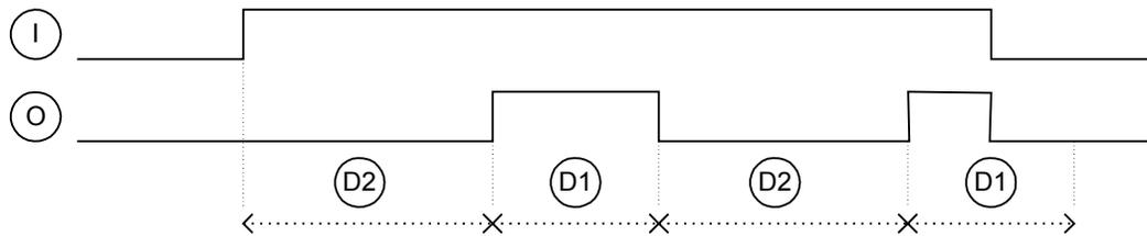
This option will also create pulses on the output but start with the delay.
