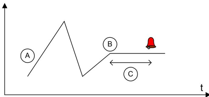
The level (A) changes constantly but at one point in time (B) it ceases to work. The sensor control will wait and see if the level changes (C) for the time set and finally generate an alarm.
