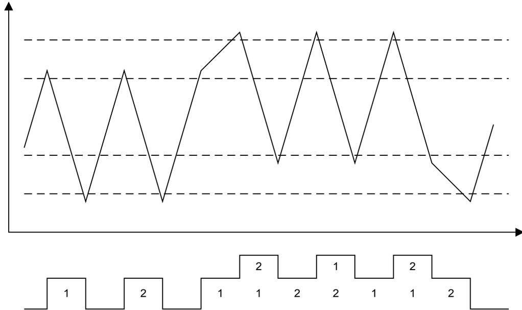
Picture showing pumping sequence when two pumps are alternated.
