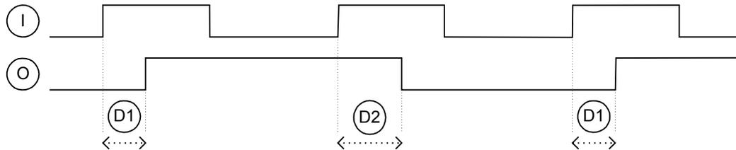
This option will create pulses on the output with half the frequency as the input.
