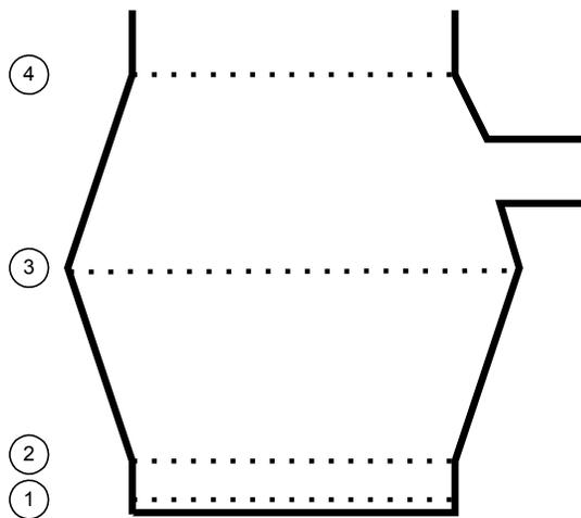
*Double-tapered pump sump with straight bottom section.*
