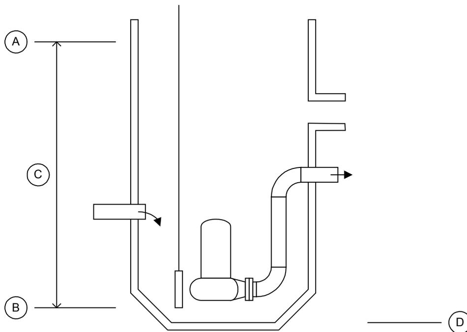
The range is specified in the max level (A) and min level (B) menus in the LEVEL group menu. The range of the sensor (C) is max level minus min level.
