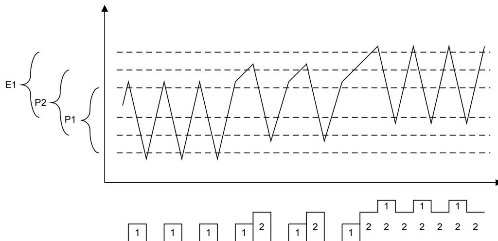
The picture shows the result. The upper part of the picture shows the changing level and the start and stop levels for P1 and P2 together with the extra start and stop level assigned to P1. The lower part shows running pumps. Two stacked numbers means that the pumps are running in parallel.
