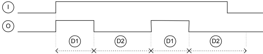
This option will create pulses on the output as long as the input is active.
