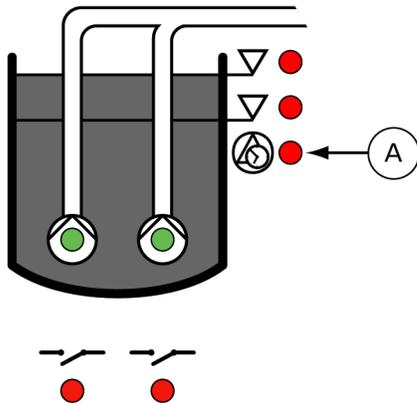
A = Capacity measurement is in progress when LED light and one ore more pumps is running.
