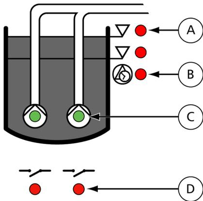
A = Indicates when the start level is reached for respective pump
