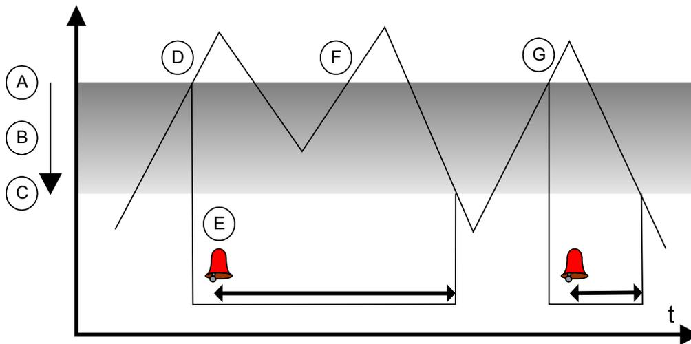
*Example of high level alarm with hysteresis and alarm delay.*
